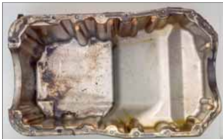
The inside of the engine oil pan was very clean. There were no sludge deposits found in the bottom of the pan.
