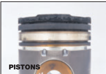
“No wear at all.”
